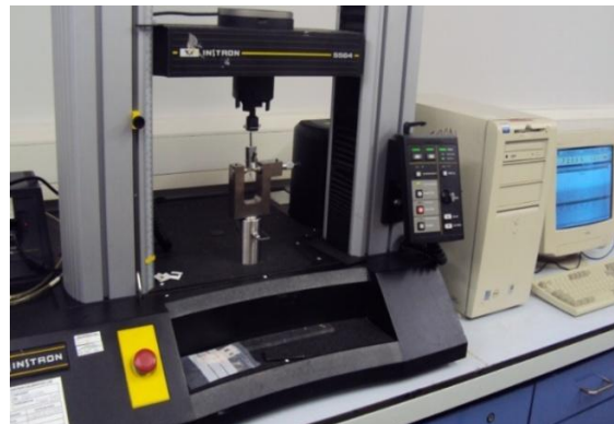
Figure 3: (a) Microbond test specimen arrangement. (b) Microbond Pull-out Testing Rig.
