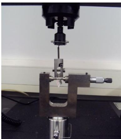
Figure 4: Close up on the microbond test pull-out grip arrangement.
